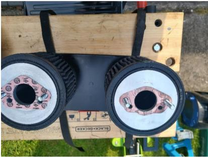
Drop the filters onto the bolts and feed two straps under each filter (you can use plastic ties not as good)
