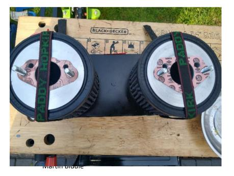
Feed the straps around to secure the filters to the faceplate
