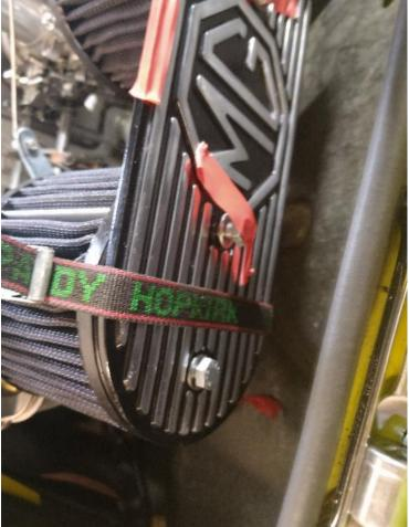
The whole filter assembly can now be lifted up and put in place
